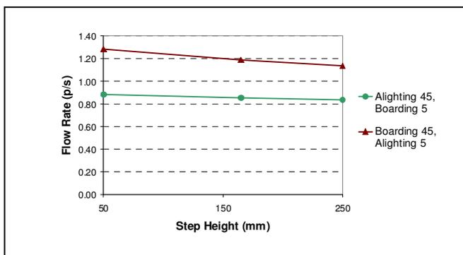
Fig. 2 Effect of vertical step distance
